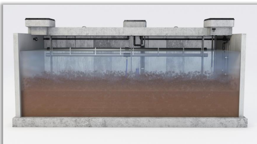
Figure 4 : SBR - Phase de décantation - Clarification
